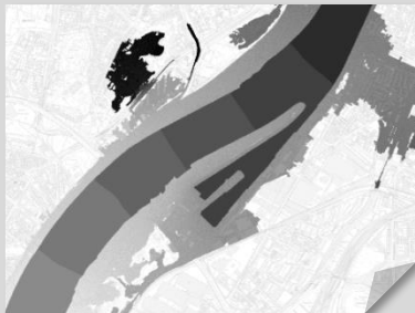
Preparation of water surface rasters from flooding levels and DTM
